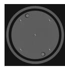
The geometric accuracy plate allows for accurate measurement of the true voxel size in the reconstructed volume. Embedded in the is an array of five tungsten-carbide beads, each 280 µm in diameter. Four beads are positioned in four corners at 35 mm apart, with one bead in the center at a distance of 24.75 mm from the other four beads.
