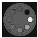
The linearity of the system can be determined using the linearity plate, which consists of vials of varying iodine concentration, covering the range of signal intensities seen in contrast-enhanced animal experiments.
