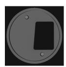
To obtain a quantitative measurement of spatial resolution, the modulation transfer function (MTF) of the system can be measured using the slanted edge method. This plate has a slanted edge consisting of a plastic-air boundary positioned at an angle of 5° relative to the CT scanner image matrix.
