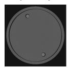
The phantom design includes a uniform polycarbonate plate positioned near the centre of the phantom to measure the uniformity and noise of the system.
